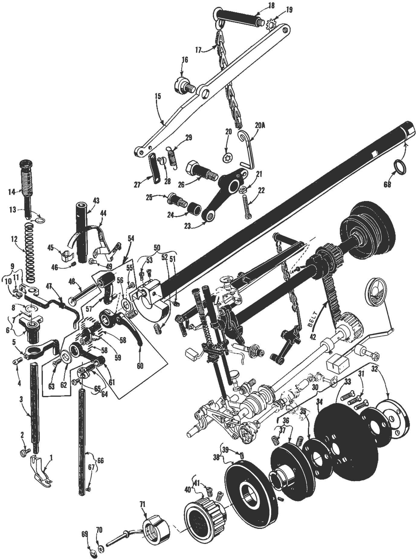
UPPER SHAFT, PRESSER BAR, NEEDLE BAR AND FOOT LIFTER MECHANISM
