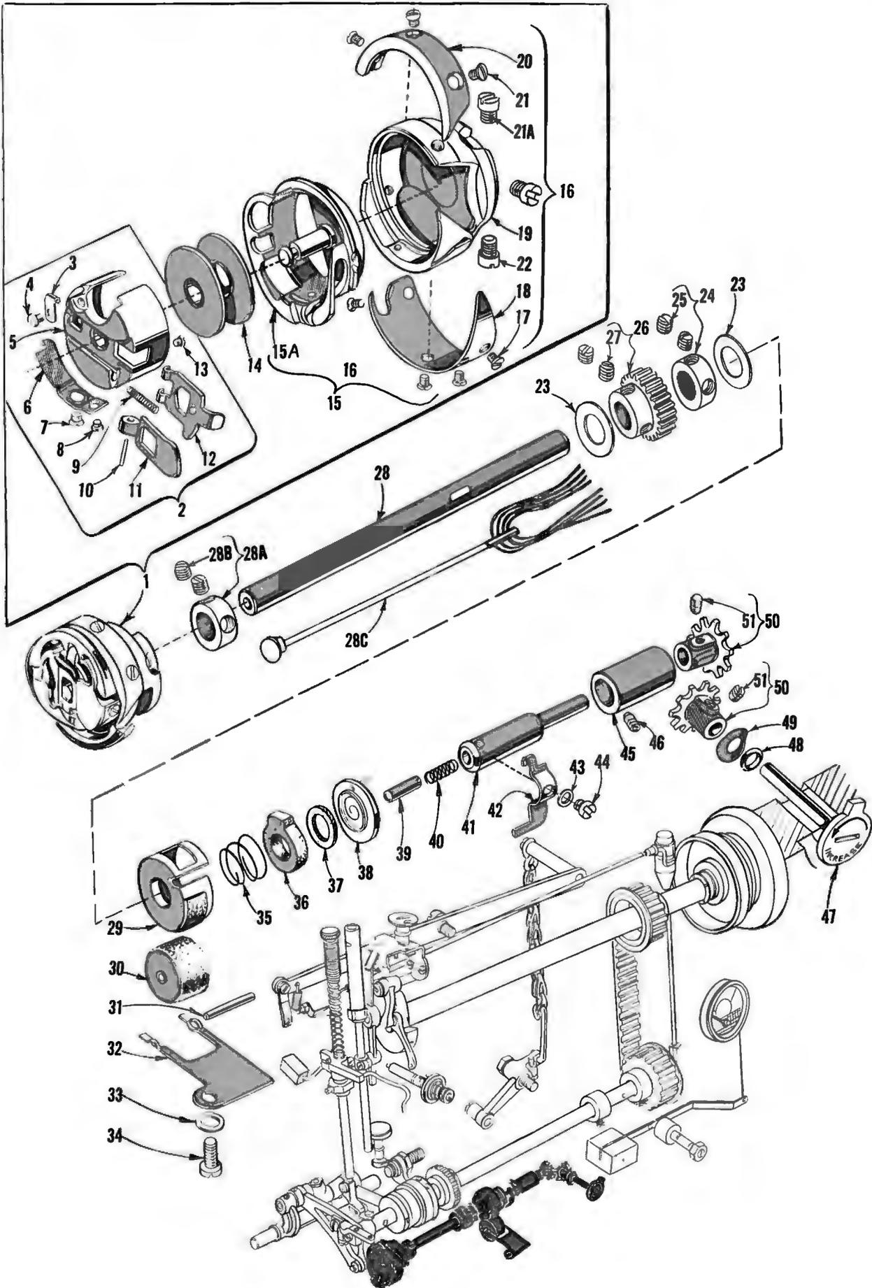
ROTATING HOOK ASSEMBLY AND HOOK OILING PARTS
