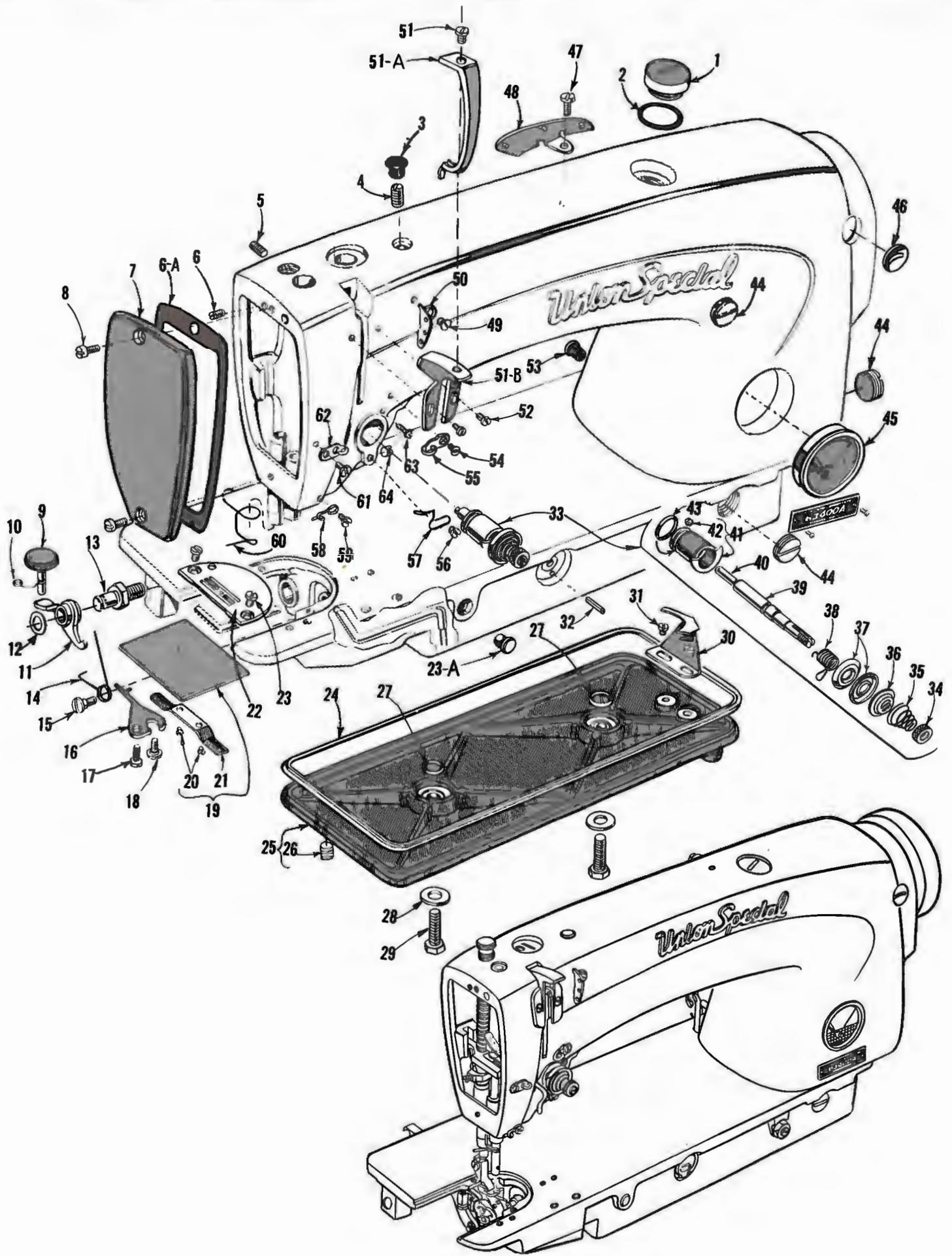
MAIN FRAME, MISCELLANEOUS COVERS AND NEEDLE TENSION PARTS
