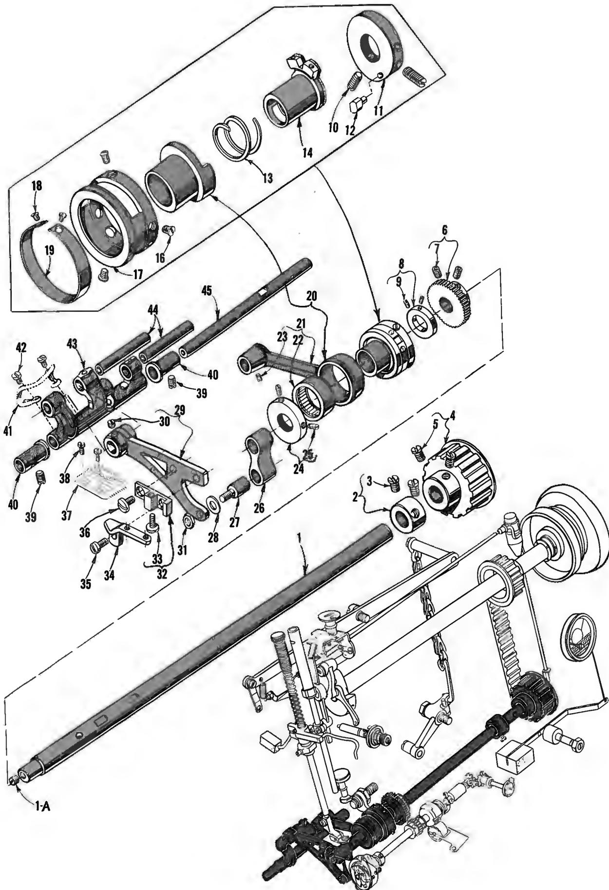
FEED DRIVING AND STITCH REGULATING MECHANISM
